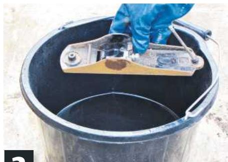
**2** After stripping down the plane, metal components are dunked in diluted Restore Pre-Clean Degreaser solution
